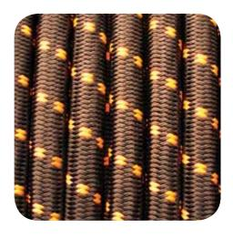
Technora aramid ropes have been engineered for applications where light weight, high strength and good abrasion resistance are important. These ropes are manufactured in a 6 strand wire lay construction with an overall jacket of polyester.
